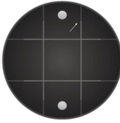
Small slots are provided in the webs around the inner perimeter of the case to locate the aerial.
