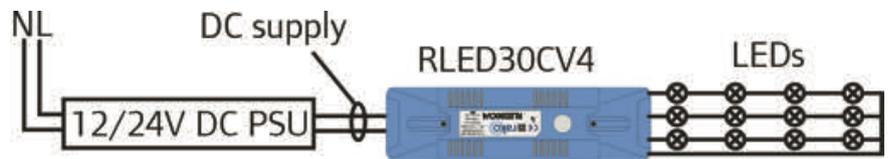
3 or 4 channel RGB constant voltage 30w/channel LED dimmer
