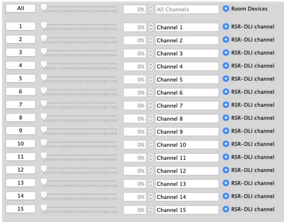
The RSR-DLI is a multi-channel device and will occupy the entire room. By default Short Address 0 will be addressed to Channel 1 in the Rako Room, DLI Short Address 1 to Channel 2 and so on for all 15 Channels.
