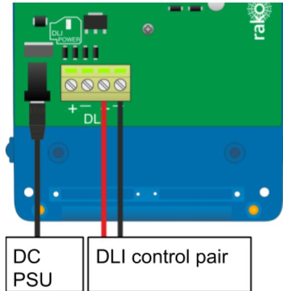
The RSR-DLI works off a 12V DC, a suitable power supply attached to a 13A plug is provided with the product. When successful powered up LED 2: the “Power LED” will illuminate.
