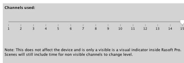
Slide the “channels used” slider to match the number of Channels required by the RSR-DLI and the remaining channels are freed up to be used by other devices.
