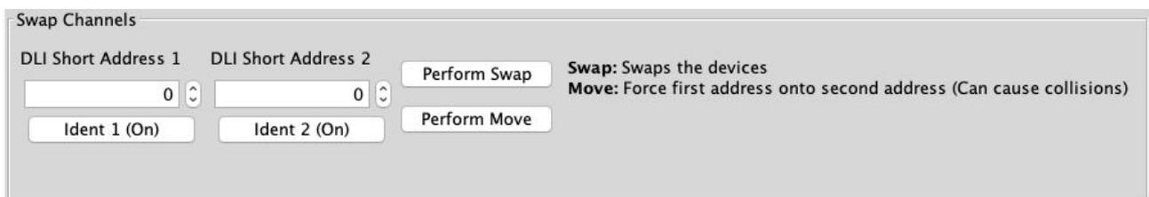
This will readdress the DLI ballast to the short address as set in each box, “Perform Swap” will directly switch the position of the two ballast. “Perform Move” will result in both ballasts having the short address of “DLI Short Address 2”.
